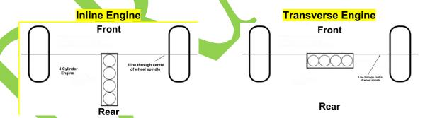
5.7.6.3 For cars with the original engine compartment at the rear of the vehicle, the engine may be moved forward, but the edge of the engine block (measured at the outer edge of the gasket), must be no further forward than a line through the centre of the rear wheel spindles. See drawing below
